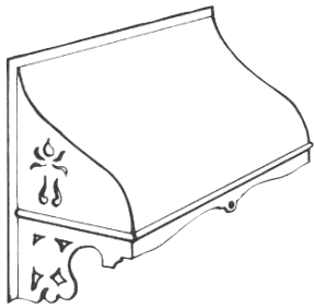
Woodworkers' Ogee No.1 Overhang 480mm Height 830mm MH1
