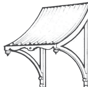
Woodworkers' Scallop With fretwork fascia and finials Overhang 565 mm Height 1300 mm WH 9
