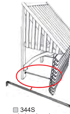
□ 344S window hood privacy screen strut stainless steel 425mm
