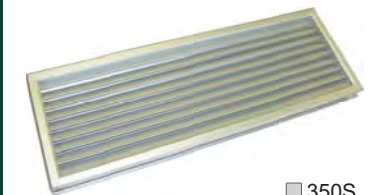
□ 350S RETURN AIR VENT aluminium 620 x 220mm cutout size: 595 x 195mm available in clear anodized and 16 powder coat colours (quantity restrictions apply)
